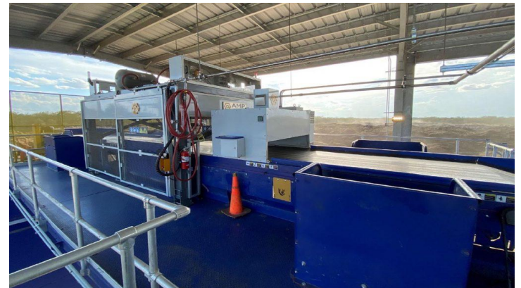
AI-equipped robot in San Antonio removes contaminants from the organics stream headed to composting
